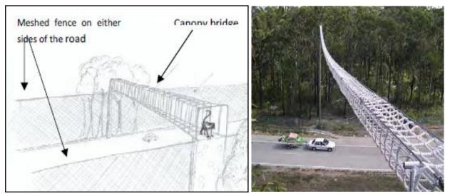
Figure 5.2: Examples of canopy bridge designs
